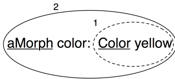
Figure 5.2: aMorph color: Color yellow is composed of two message sends: Color yellow and aMorph color: Color yellow.
